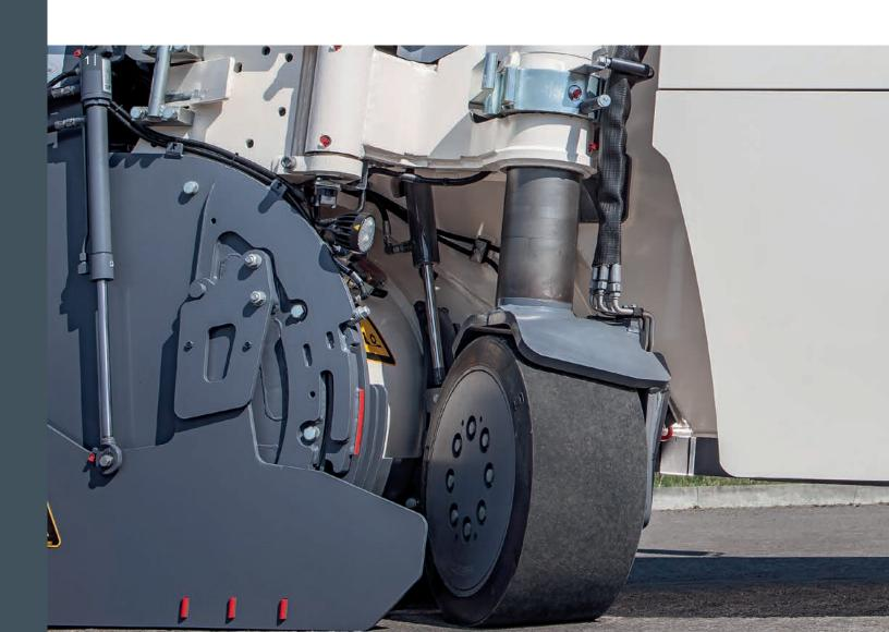
1 The machine's extremely large locking angle facilitates operations on construction sites offering limited space.
