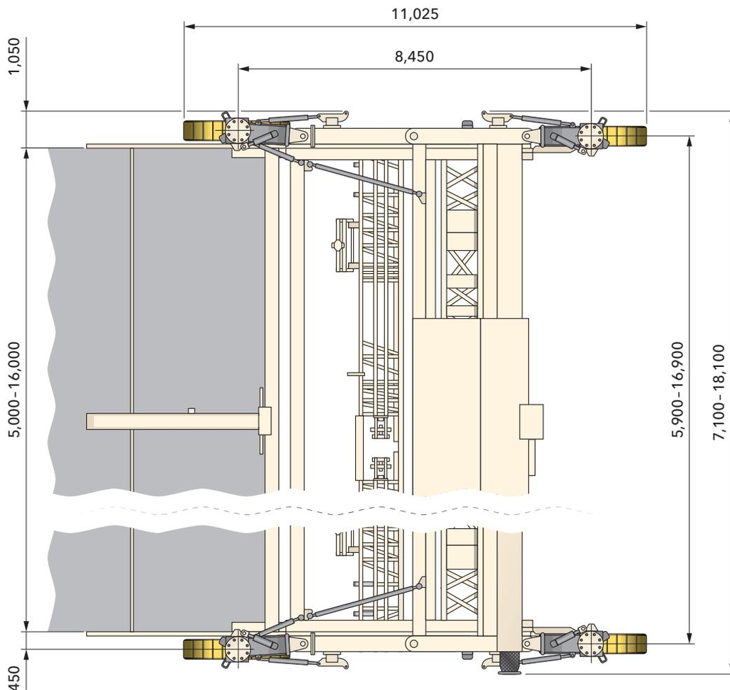
Slipform paver SP 1600 for dual-layer concrete paving operations equipped with dowel bar inserter, longitudinal joint tie bar inserter, oscillating beam and super smoother
